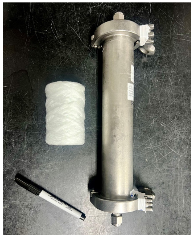
Glass fiber filter (left) for solid phase analysis. Stainless steel column (right) contains resin beads for dissolved phase extraction.
