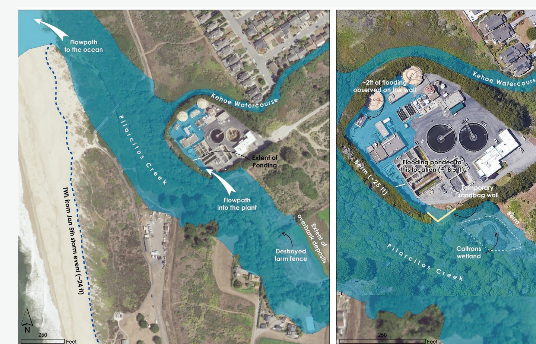
Figure 7. Representation of flooding extents during December 31 storm derived from deposits, photos, and observations of high water
