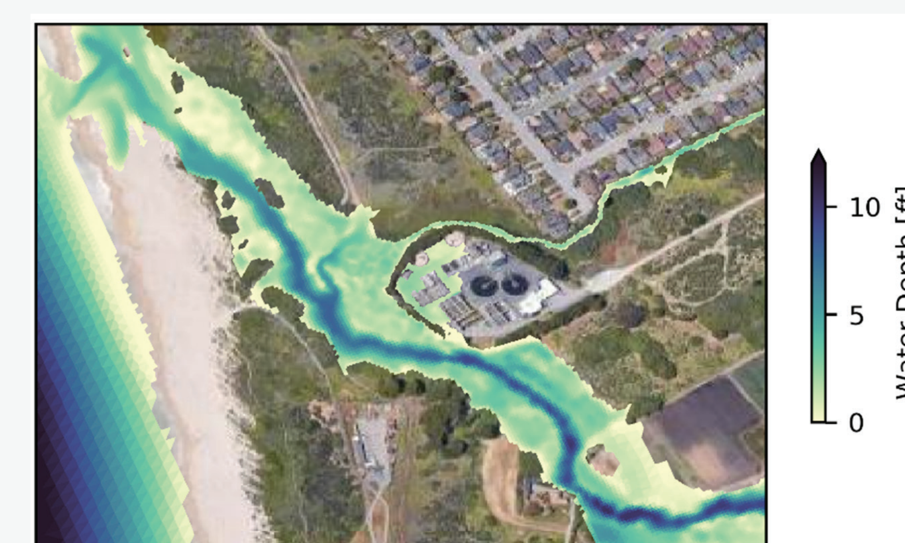
Figure 8. DFlow-FM model results for the December 31 storm. The model reproduced observed flood depths to within a few inches at key facility locations
