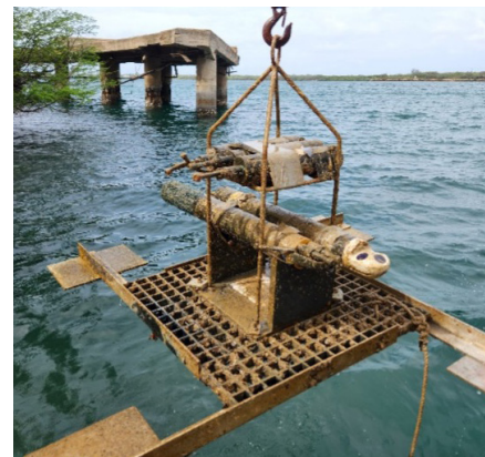
OPTICS instrumentation system deployed at the base of Oscar 1 Pier Outfall in DU N-2, Pearl Harbor.
