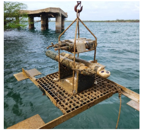
OPTICS instrumentation system deployed at the base of Oscar 1 Pier Outfall in DU N-2, Pearl Harbor.
