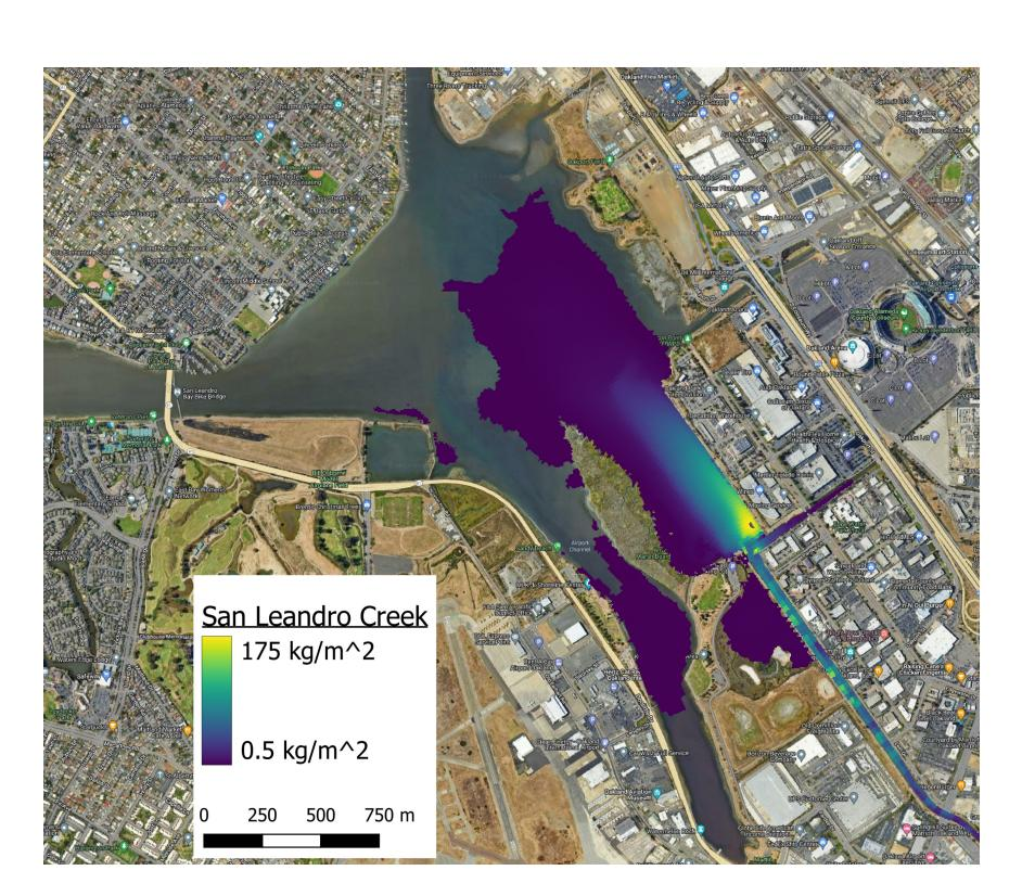
Left: Sediment deposited on bed after 1 year from Peralta Creek | Right: Sediment deposited on bed after 1 year from San Leandro Creek
