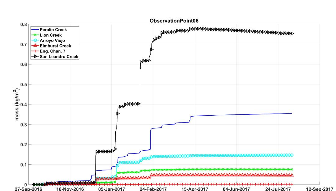
Left: Sediment mass at eight locations in San Leandro Bay from six different watershed inputs after 1 year | Right: Sediment deposited over time in center of SLB
