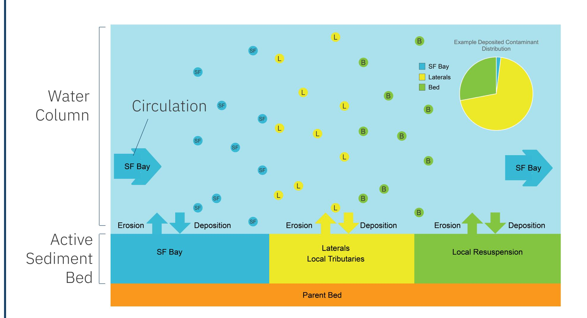
Conceptual diagram of SLB sediment sources
