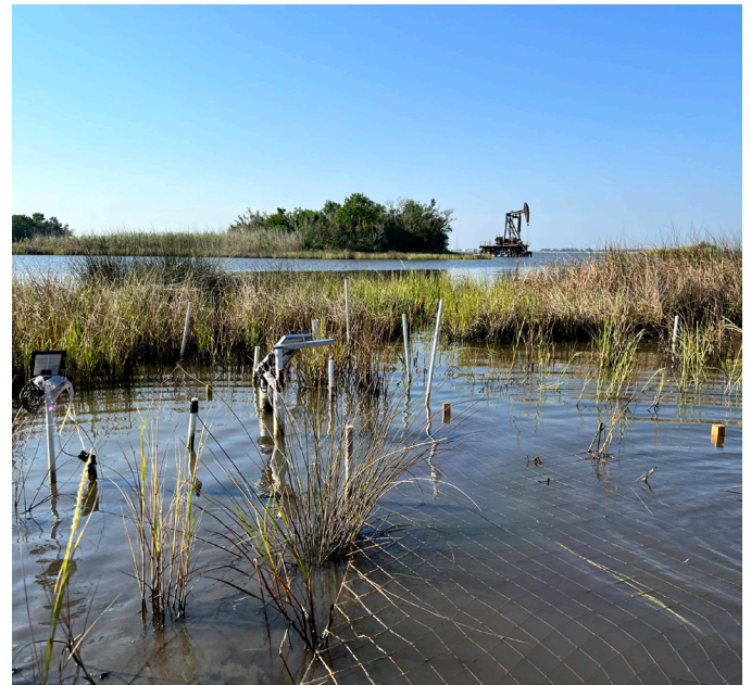
Twine-mesh grids supported S. alterniflora transplants in ponded areas. The plot soils are aerated by fertilizer application PVC tubes and solar-powered aeration pumps.
